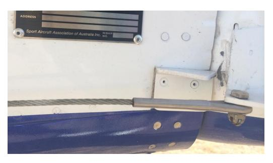
Lower photo shows the correct (albeit unfinished) installation using the correct (fork) end fitting at the Rudder.
