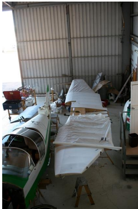
Bottom covering done. Two panels on top surface covered and shrunk, one covered and awaiting shrinking, one about to be covered
