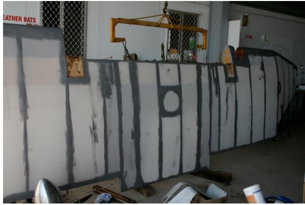
First coat of sun barrier, a single pack polyurethane, brushed on over the framework to bond the cloth to the frame
