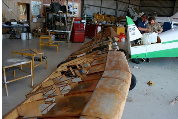
Dismantled, stripped, ready for a light sanding and varnish as soon as the wheels are off
