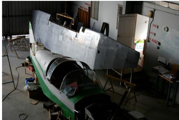
Full coat of sun barrier applied, awaiting top coat
